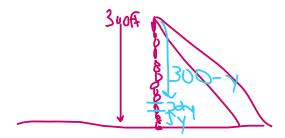
How much does the little segment of the chain weigh? Weight=force=dy\*density=5dy How far is the segment being moved? 300 - y
