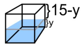
For a slice at height y, the distance the water has to be moved is 15 feet, minus the distance it started at
