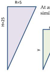
At any height in the tank, the filled portion of the tank forms a similar triangle with the triangular profile of the entire tank.
