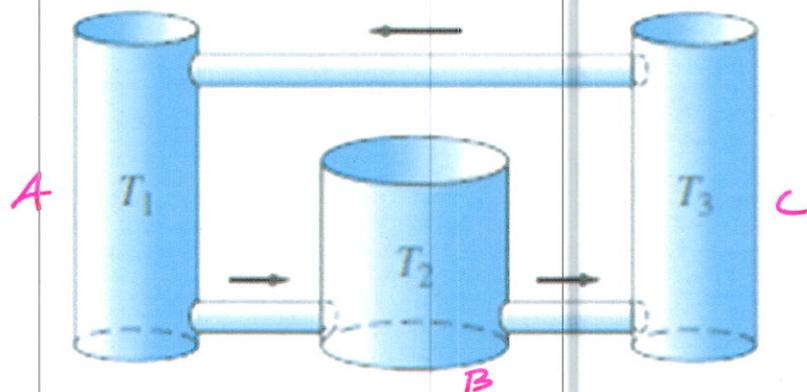
(Tank 1 feeds into Tank 2; Tank 2 feeds into Tank 3; Tank 3 feeds back into Tank 1.)
