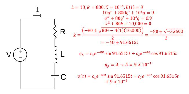
Underdamped Graph shown with arbitrary constants since there are no initial conditions Long term:  $9 \times 10^{-5}$  steady state.
